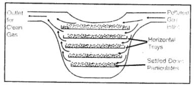
Gravitational Settling Chamber
